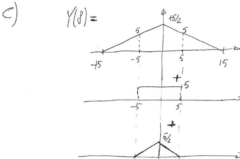
$$y(t) = \frac{1}{2} \left( \frac{\sin \pi 15t}{\pi t} \right)^2 + 5 \cdot \frac{\sin \pi 10t}{\pi t} + \frac{1}{2} \left( \frac{\sin \pi 5t}{\pi t} \right)^2$$
