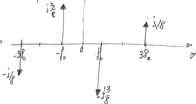
$$f_{\max} = 3f_0 \quad f_s > 6f_0 \quad T < \frac{1}{6f_0}$$
